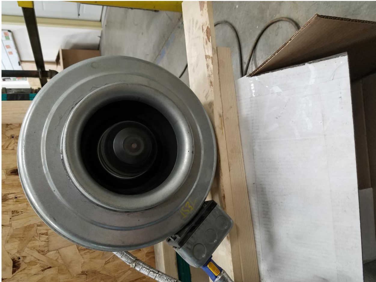
Picture 7 – Blaze 6 I/O Glass Cooling Intake Fan
